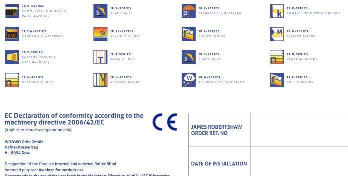
Intended purpose: Awnings for outdoor use Corresponds to the provisions set forth in the Machinery Directive 2006/42/EC if featuring a motor drive. The following standards are applied: EN 13651 External blinds – Performance requirements including safety EN 60335-2-97 Household and similar electrical appliances – Safety EN 12045 Shutters and blinds, power-operated Conformity with the following Directives: Electromagnetic Compatibility Directive 2004/108/EC
